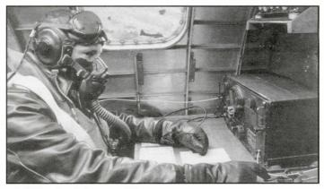
in front of him. The liaison radio receiver and transmitting key were located on the radio operator's table, while the liaison radio transmitter was mounted to the bulkhead directly behind him.
